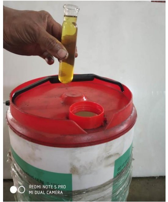
Take Oil Sample in Test Tube
