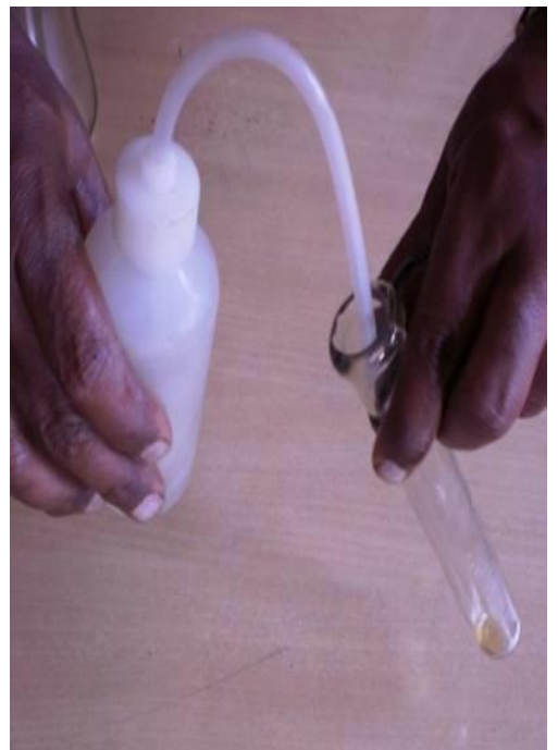
Clean all glass ware with Petroleum Ether ( Do not use Cloth or other Medium for Cleaning
