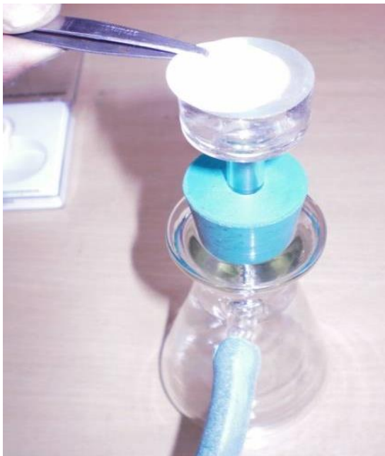
Place Test Patch on Porous Base
