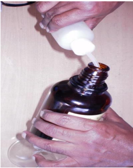
Take Petroleum Ether in Flushing Bottle
