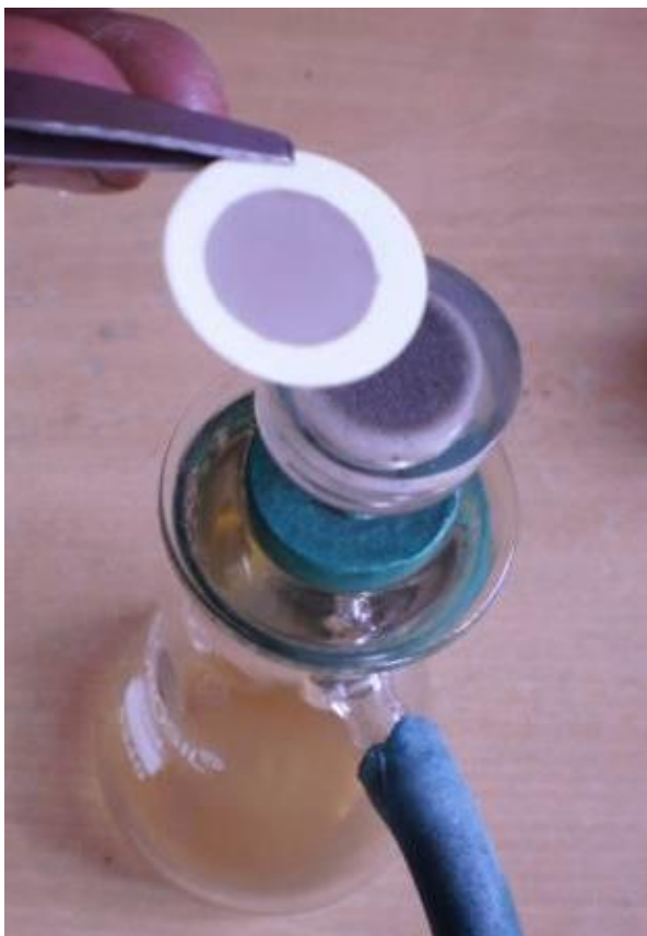
Take Out Test Patch Carefully
