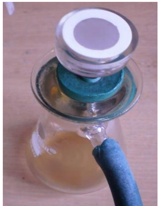
Remove Glass Funnel from Porous Base
