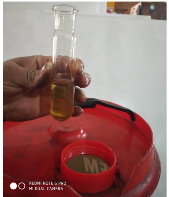
Take Oil Sample in Test Tube
