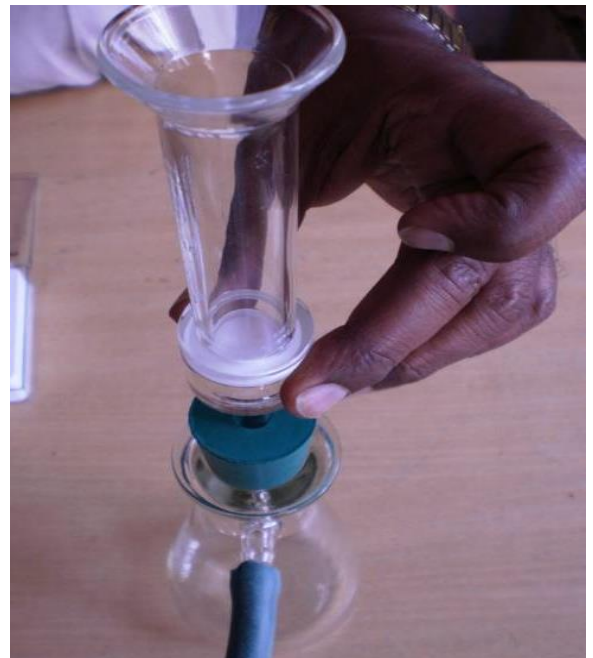
Place Glass Funnel on Porous Base
