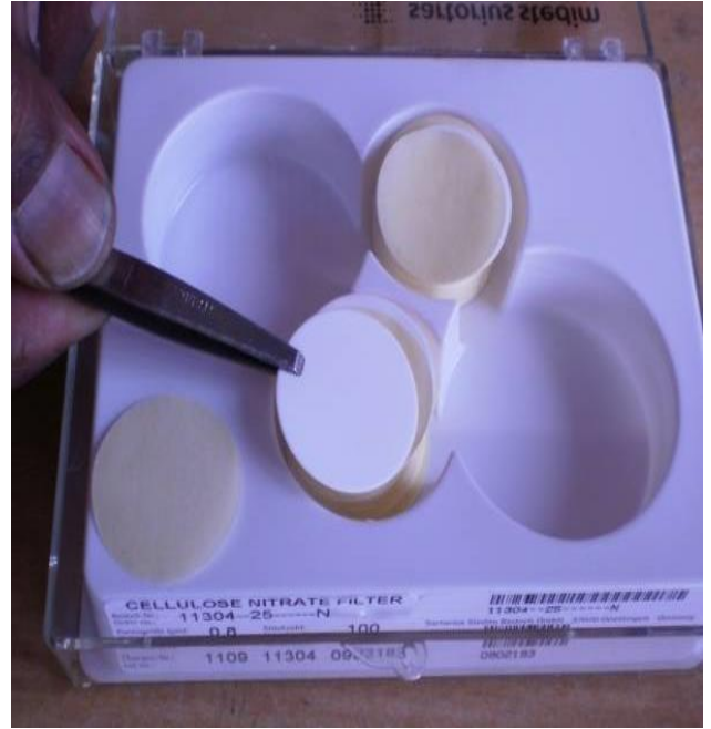
Carefully Lift Test patch. (discard the blue Cover paper)
